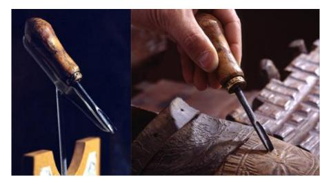
**6 Auger** 1987.29.68 To hollow out the inside of the sabot.
