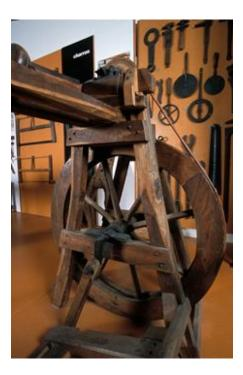
**1 Lathe** 1987.31.31 For turning wooden parts (box of cartwheel).
